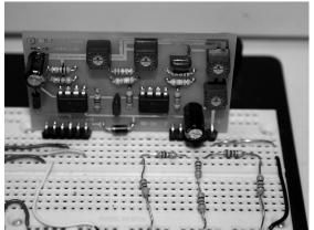
If you are using the *Phase Tripler II* board, handle it by the edges and carefully insert it into the breadboard. Connect the power supply ground and function generator ground to pin 2, function generator signal to pin 1, +12VDC to pin 4, and -12VDC to pin 6.
