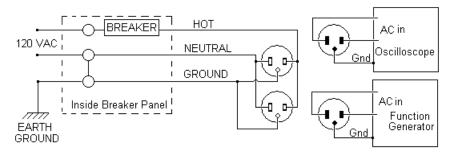
Note that the wide connector on the receptacle and the ground connector are connected together and to earth ground at the breaker panel. So the function generator and oscilloscope grounds are connected together through the AC power outlets.
