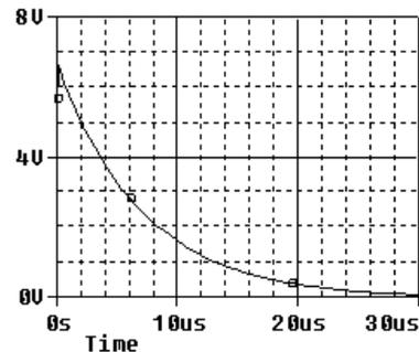
$V_P$  is the peak amplitude at  $t$  equal to zero. The decay rate,  $\alpha$ , is the reciprocal of its time constant. Its impulse function can be expressed as:  $45.5\delta(t)$ .
