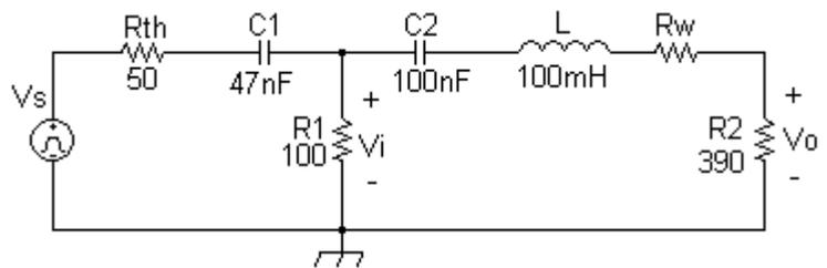
4. Connect channel 1 across  $R1$  to measure  $V_i$ . Expand the display for best accuracy.
