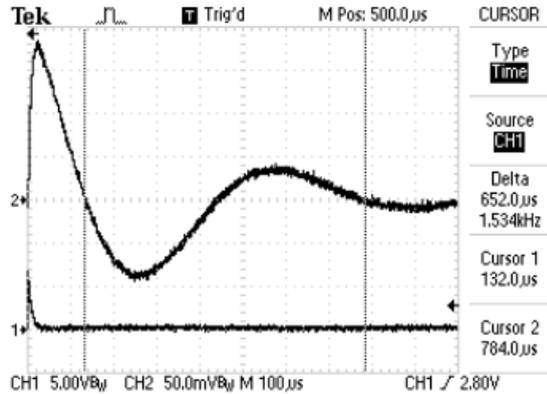
Note the pulse on channel 1 and its timing relationship to the RLC response on channel 2.
